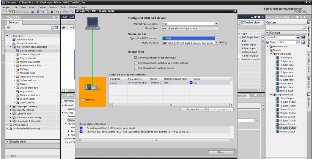
Click on “Go online”. Check the status in TIA portal to analyse if the configuration of the PLC and the Machine Vision Device fit together.
