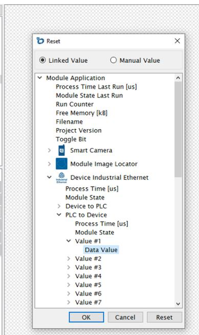
The screenshot shows the 'Reset' dialog box. The 'Linked Value' radio button is selected. The tree view in the dialog is expanded to show the 'PLC to Device' module, with 'Data Value' selected under 'Value #1'. The 'Reset' button is highlighted.
