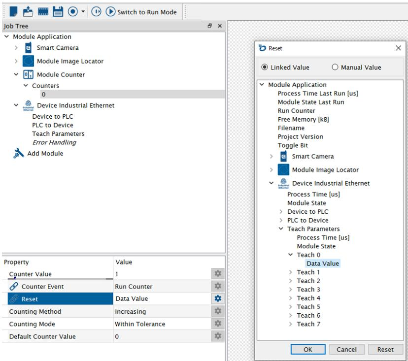
The screenshot displays the software interface. On the left, the Job Tree shows a hierarchy: Module Application > Smart Camera > Module Image Locator > Module Counter > Counters > 0 > Device Industrial Ethernet > Teach Parameters. The 'Reset' parameter is selected in the 'Property' table below the Job Tree.
