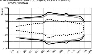
Characteristic curves show the position of the center or the front edge of the measured object (100  $\times$  100 mm plate) at the time of switching. U2GT002/U2GT004
