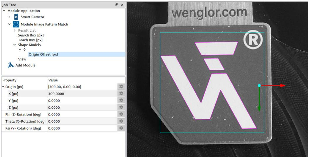
The Sub-Module View allows to activate or to deactivate certain UI elements for found objects (contour, coordinate system, extension lines of coordinate system).
